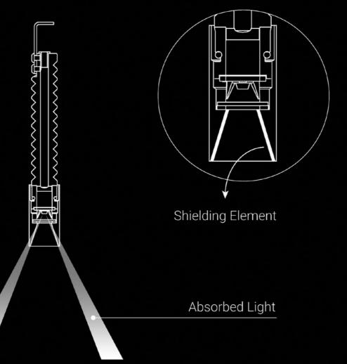
The Extradark system associates an optical TIR PMMA lens to an element that geometrically shields the light beam viewing angle to obtain highly uniform lighting and full beam control.
