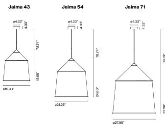
Jaima 43 LED COB 13.5W 2700 CRI90 Luminaire 529lm Light Source 1092lm (included) Jaima 54 LED COB 13.5W 2700 CRI90 Luminaire 514lm Light Source 1092lm (included)
