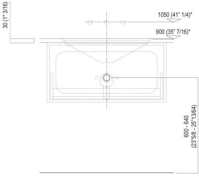
Scarico per sifone a bottiglia e ad incasso Drain for bottle trap and concealed waste trap
