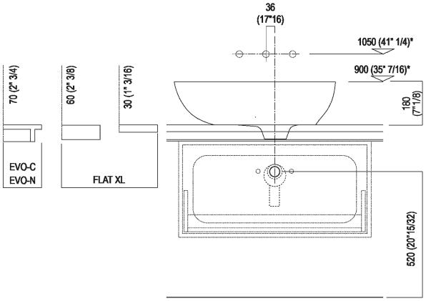
Scarico per sifone a bottiglia e ad incasso Drain for bottle trap and concealed waste trap
