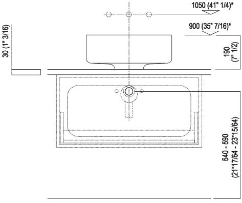
Scarico per sifone a bottiglia e ad incasso Drain for bottle trap and concealed waste trap
