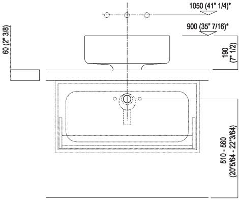
Scarico per sifone a bottiglia e ad incasso Drain for bottle trap and concealed waste trap
