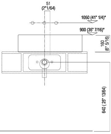
Scarico per sifone a bottiglia e ad incasso Drain for bottle trap and concealed waste trap
