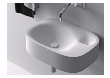
Wall mounted washbasin in white Cristalplant® biobased with overflow hole in a small basin connected with the main basin, which also can be used as a soap holder. Wall mounted version with or without tap hole. Designed for waste .MET0563. Fixing kit included. The overflow hole has a maximum capacity of 8 l/min, therefore it is advisable to install a waste designed for washbasins without overflow.
