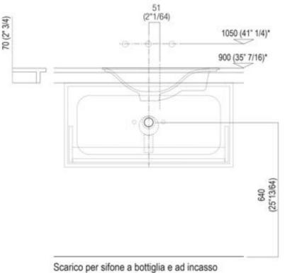
Drain for bottle trap and concealed waste trap
