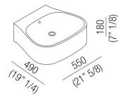
Shaped ceramic washbasin available in white, in two colours (with grey external surface RAL7021) or with grey floral motif. Supplied either with one, three or without tap holes; with overflow hole complete with polished stainless-steel overflow collar and fixing kit. Designed to take waste .MET0346P or .MET0562.
