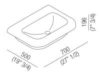
Washbasin in white or two-coloured Cristalplant® biobased (exterior in dark grey RAL7021 or light grey RAL 7044), without tap hole, or with 1 or 3 holes for tapware units. Without overflow, fixing kit included. Designed for waste .MET0563. The washbasin is available in customized colours (surcharge of 20%).
