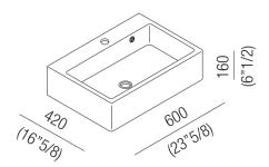
Rectangular washbasin made from Cristalplant® biobased with holes to take mixer tap. Complete with overflow, polished stainless-steel overflow collar and fittings, including fixing kit. Designed for waste .MET0346P or .MET0562.
