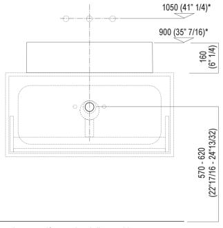
Scarico per sifone a bottiglia e ad incasso Drain for bottle trap and concealed waste trap
