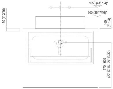
Scarico per sifone a bottiglia e ad incasso Drain for bottle trap and concealed waste trap
