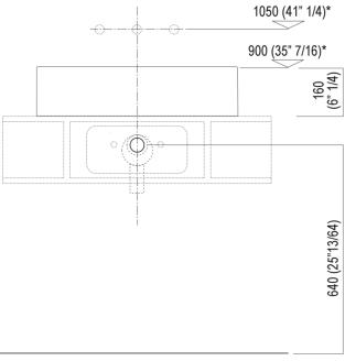
Scarico per sifone a bottiglia e ad incasso Drain for bottle trap and concealed waste trap
