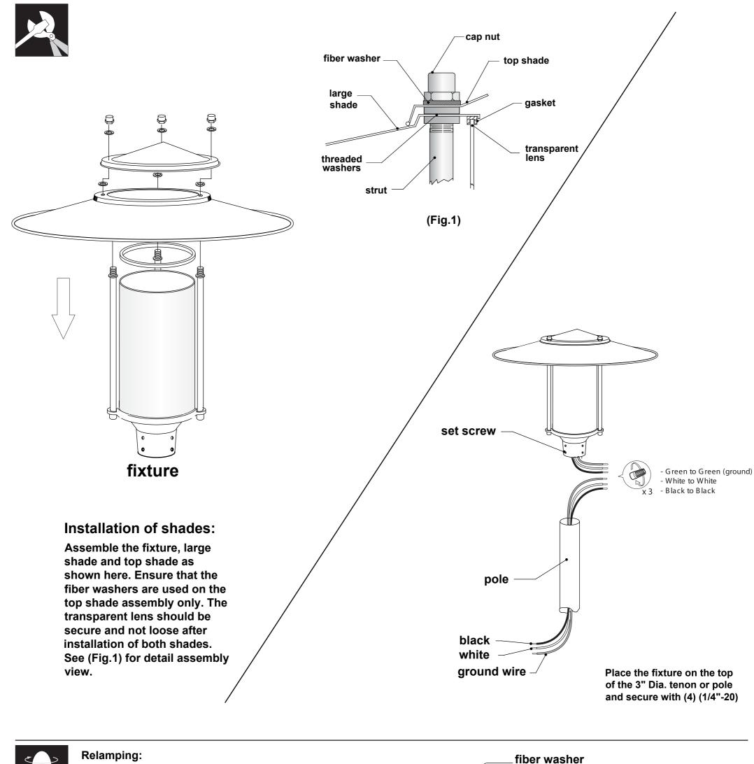
Remove cab nuts, fiber washers and top shade. Install lamp (light source) as specified.
