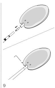
Plug the lamp into lamp socket. Ensure power to lamp is working correctly.
