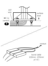
After each branch is installed, feed pull wire through pre-laid conduit to the driver (power: is no interference with adjacent branches, supply) location.
