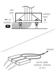
After each branch is installed, feed pull wire through pre-laid conduit to the driver (power: is no interference with adjacent branches,
