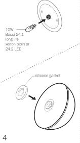
Lamp fixture using Bocci 24.1 long life bipin xenon lamp, or Bocci 24.2 LED.
