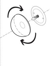
Gently thread cast glass hemisphere onto cover plate. Do not tighten past the point of contact.
