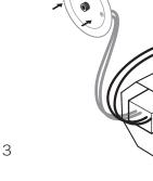
Slightly stretch the silicone ring to fit around the cover plate.
