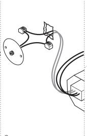
Join transformer wiring to cover plate wiring using connectors provided.
